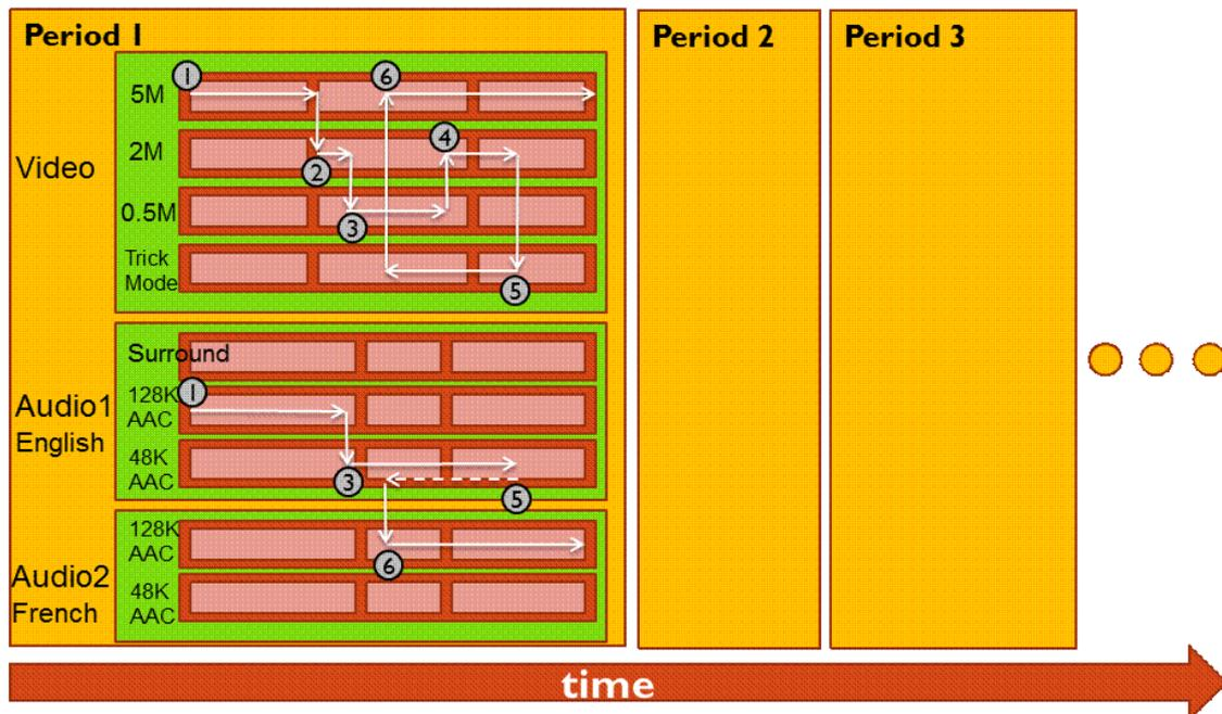
Figure 1. A simple example of dynamic adaptive streaming. Numbered circles demonstrate the action points taken by the device.
